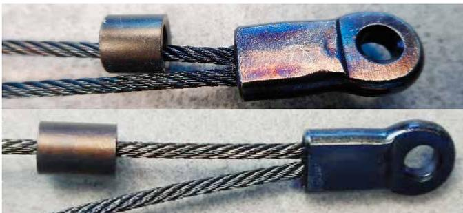
Picture 1: Examples of different color effects on the different materials rope, sleeve and eyelet
